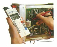
Input resistance exceeding  $10M\Omega$ Input resistance for both AC and DC in the voltmeter is in excess of  $10M\Omega$  so that small amounts of voltage in transistor circuits, etc., can be measured without adversely affecting the condition of the circuit.
