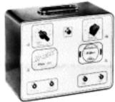
Heterodyne Marker-adder. Provides a conti marker (including trap points) that will not al receiver's response curve. Functions with a marker and sweep equipment that has an outp 0.05 volts or more. Complete with leads. S
