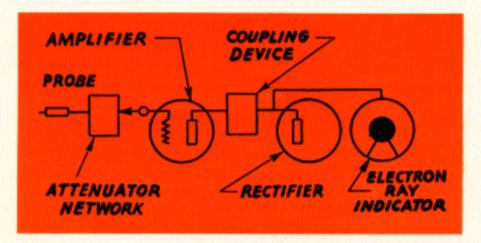
The a-f channel employs three tubes: an amplifier, a diode rectifier and an electron-ray indicator. It is resistance-
