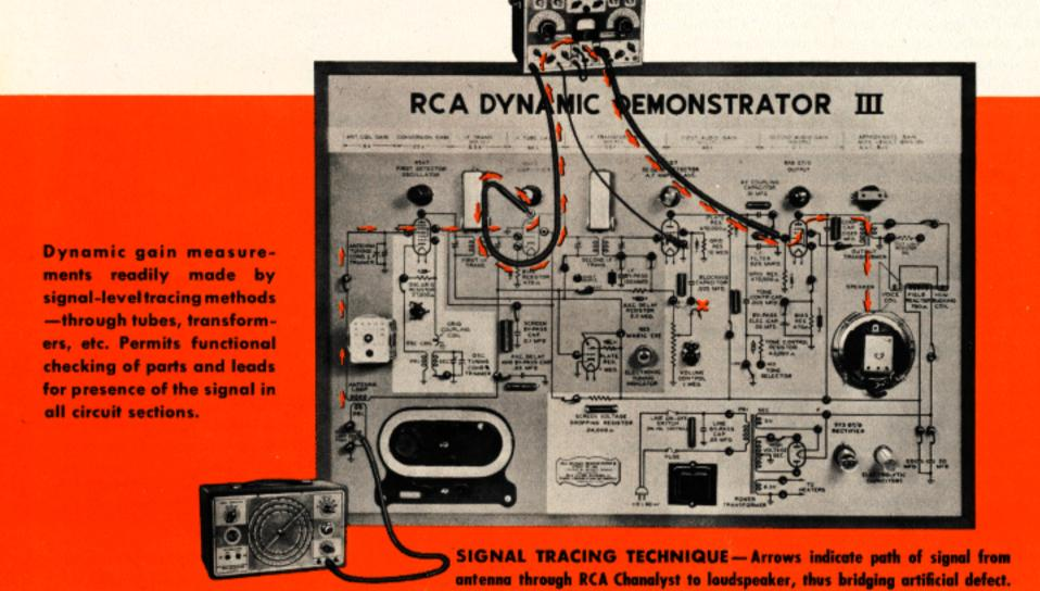
If you want to listen to the signal in ANY part of the radio receiver, you can do so with the RCA Chanalyst. Simply plug in a pair of high-impedance headphones... or connect the output of the audio channel to the last receiver tube and speaker and you will be able to HEAR the signal picked up by the Chanalyst probes. By tuning in a local broadcast station and following its signal through the receiver you can locate quickly the precise stage where
