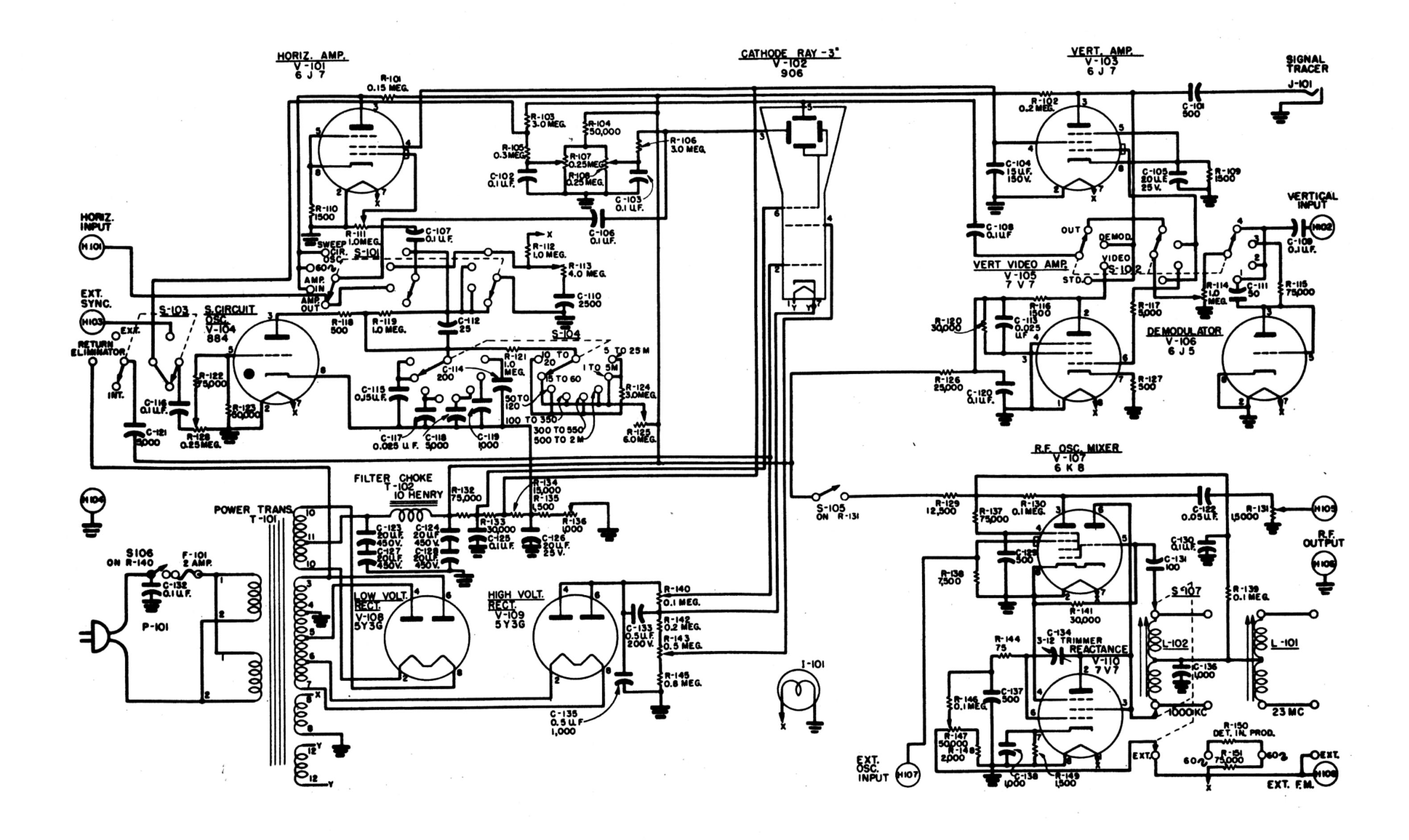
Fig. 22-31.—Schematic of Hickok Model RFO-5.
