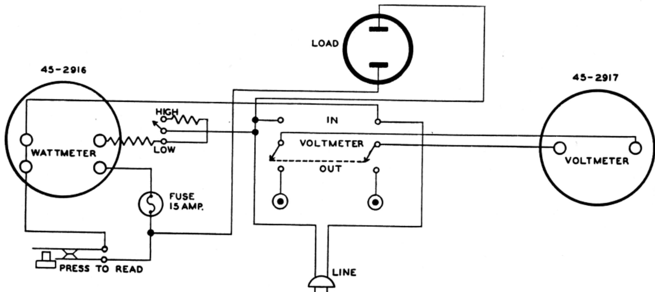
PHILCO MODEL 029 APPLIANCE TESTER (SCHEMATIC DIAGRAM)
